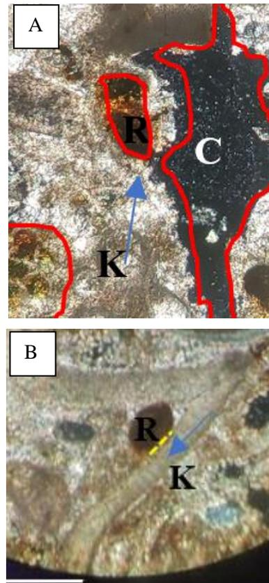
Figure 9. Compaction process between point contact grains in sample C3 (top) and long contact in sample C4 (bottom).
