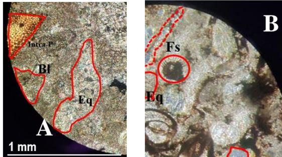
Figure 5. Equant cement (Eq), Bladed cement (Bl) in sample C2 (A) Fibrous cement (Fs) in sample B1 (B)
